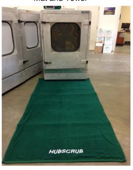
A vinyl mat on the floor surface and terry cloth towel on top is used to contain drips of water when the door is opened or from equipment when removed. It is 4' wide by 8' long. Both the mat and towel has Velcro sewed in along the sides which can be separated at the end of the day to be dried or washed and dried.
