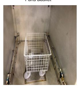
The parts basket is 11" high X 20" long by 16" wide. Swivel caster wheels are 5 inches high to raise the basket off the floor for the underspray and for mobility convenience. Excellent cleaning is achieved by the underspray system and the rotating spray systems that provide spray pressure to all sides of the parts.
