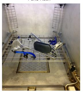
Our parts rack is stainless steel and can accommodate 50 + lbs. The rack has six hooks that rest on the guard rails and is very easy to install and remove. The rack measures 30" X 30" providing ample room for all types of parts. This photo shows a small sample of parts. Once again the combination of the underspray system and rotating spray systems provide deep cleaning and disinfection for all sides of the parts.
