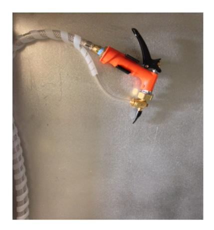
The Personal Spray Attachment is very handy and recommended for all models. The attachment is located in the front corner as you open the door so it can be quickly accessed. It can dispense a detergent for washing equipment and also includes a rinse function providing a complete cycle for equipment that does not need the full *HUBSCRUB* cycle, Spray pressure is govern by the facility water pressure. The system does not need power to operate the Spray Attachment.
