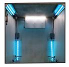
The effectiveness of UV depends on: a clean surface, distance from the UV lamp to equipment surface, how long the lamps are on and a direct line of sight to the equipment surface. These important requirements is why **HUBSCRUB UV** is so effective and quick.
