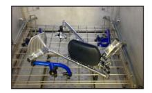
**Parts Basket** is 11" H X 20" L X 16" W. Swivel casters are 5" high to raise the basket off the floor for the underspray. Caster wheels are convenient to roll the basket to **HUBSCRUB**.
