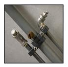
This photo shows three spray nozzles that are mounted on the rotating spray arms. The dark nozzle in the middle is used for washing and rinse cycle and is 1 of 12 nozzles. The nozzle on the right side of the middle nozzle is used by the concentrate disinfectant. The nozzle on the left size of the middle nozzle is used by the Ready To Use (RTU) Disinfectant.
